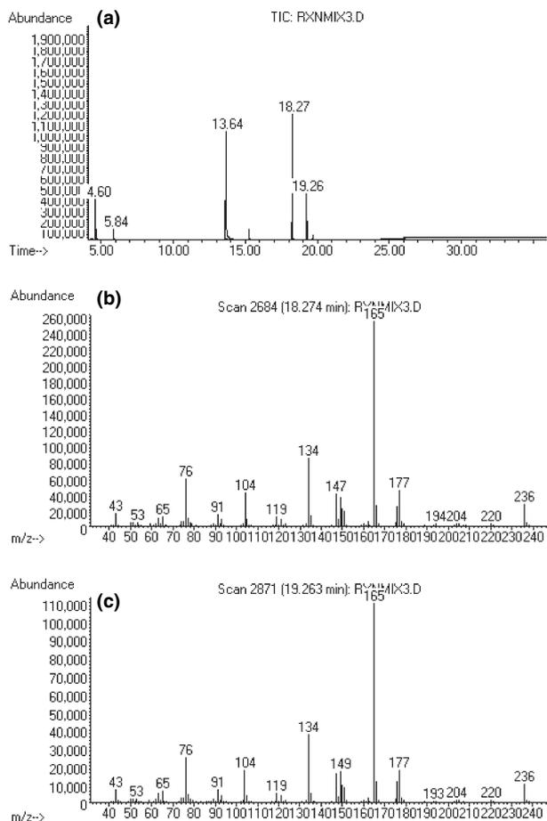
FIG. 5—Total ion chromatogram (a) and mass spectra (b and c) of the reaction mixture resulting from the synthesis of methyl 3-[3',4'-(methylenedioxy)phenyl]-2-methyl glycidate using the method of Elks and Hey (4).
