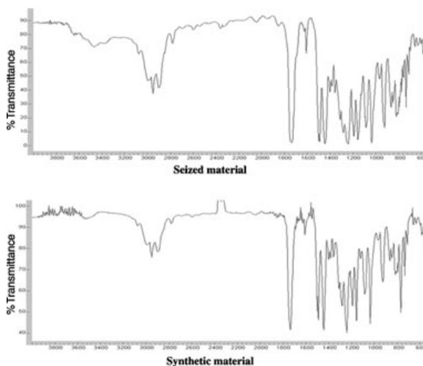
FIG. 6—Infrared spectra of the seized material (a) and the synthetic methyl 3-[3',4'-(methylenedioxy)phenyl]-2-methyl glycidate (b).
