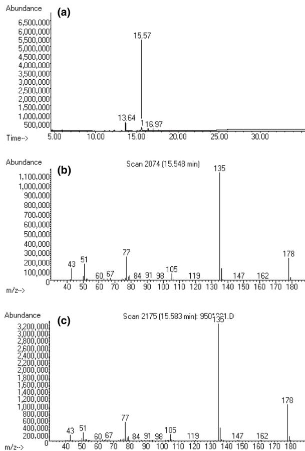
FIG. 4—Total ion chromatogram (a) of the hydrolysis and decarboxylation product obtained from the seized material; mass spectrum (b) of the chromatographic peak at 15.57 min; mass spectrum (c) of a certified reference standard of 3,4-MDP2P.
