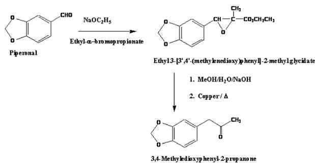
FIG. 2—Reaction pathway from piperonal to 3,4-MDP2P via ethyl 3-[3',4'-(methylenedioxy)phenyl]-2-methyl glycidate.
