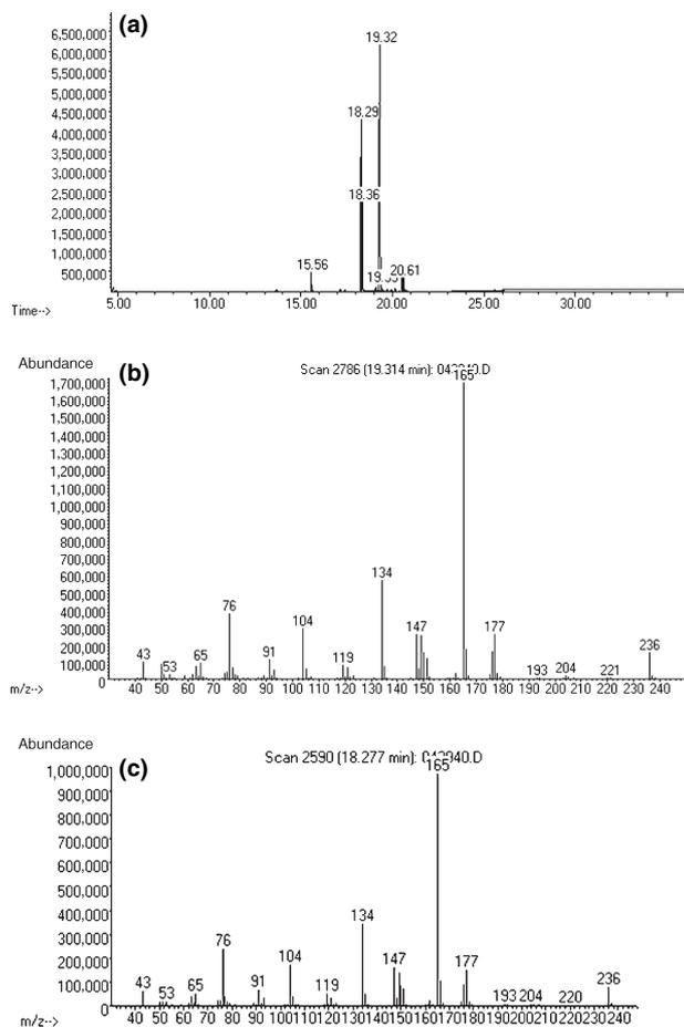
FIG. 1—Total ion chromatogram of the seized material (a) and mass spectra obtained from chromatographic peaks at 18.29 (c) and 19.32 min (b).
